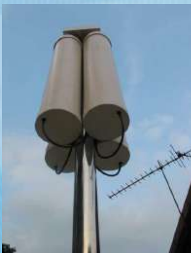
Development of wifi antenna for transmitting information up to 3 km
