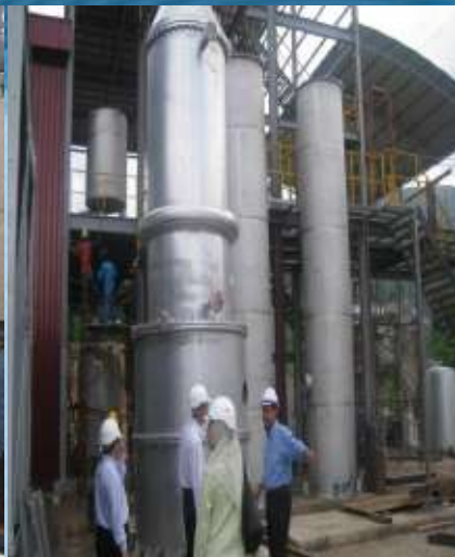
Pilot Plant for production of water-soluble polymer for industrial waste treatment
